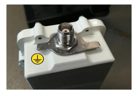
Besides the mains voltage safety, proper grounding is essential also for the error free operation of radio links and the protection against over-voltage and lightning. Although SATEL Proof radio modem incorporates a robust internal surge protection, the surge spikes and power transients caused by lightning, ESD or other electrical systems must be discharged to earth ground.
