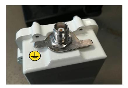
Besides the mains voltage safety, proper grounding is essential also for the error free operation of radio links and the protection against over-voltage and lightning. Although SATEL Proof radio modem incorporates a robust internal surge protection, the surge spikes and power transients caused by lightning, ESD or other electrical systems must be discharged to earth ground.
