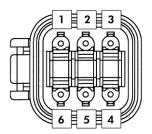
Pin-out of Deutsch DT04-6P-CL09 power/data connector
